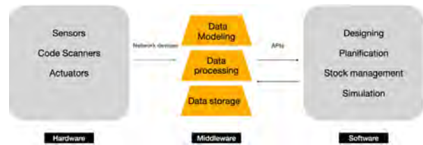
Figure 2. System architecture based on a digital twin concept from Altexsoft [9]
